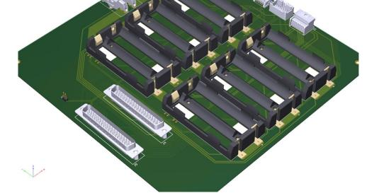
Fig. 4: Battery Board, where our battery cells and all connections to them will reside
