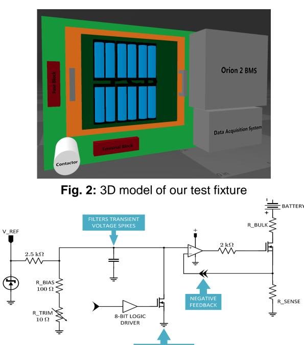
Fig. 3: Load Profile Circuit
