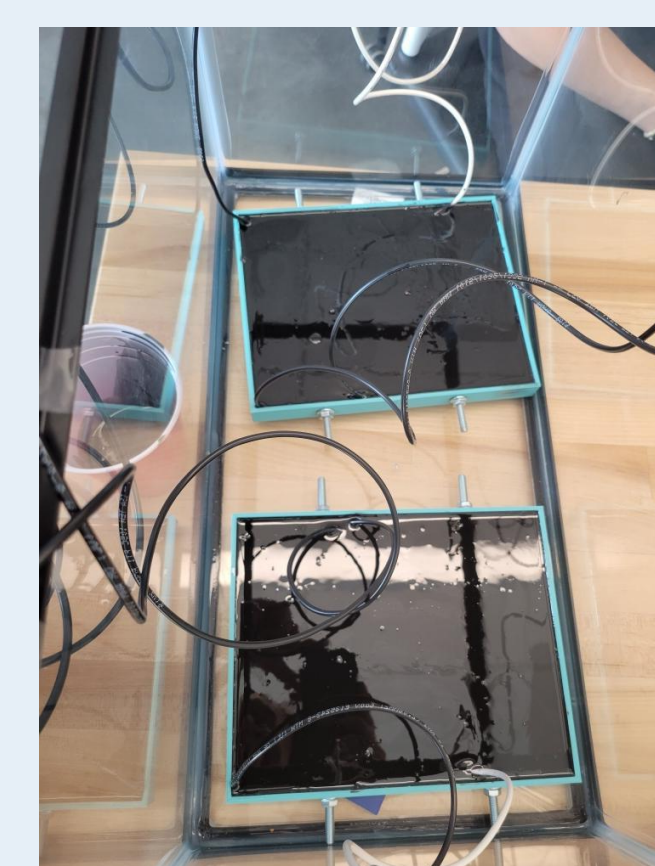
Fig. 3: Primary and secondary coils potted
