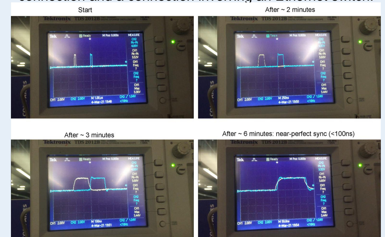
Fig. 4: PTP synchronization process shown on an oscilloscope
